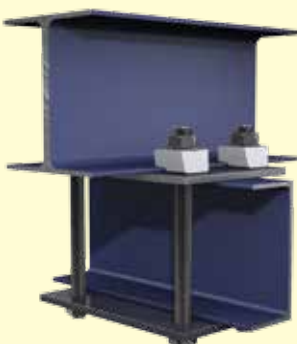
Channel section below I-Section at 90 degrees
