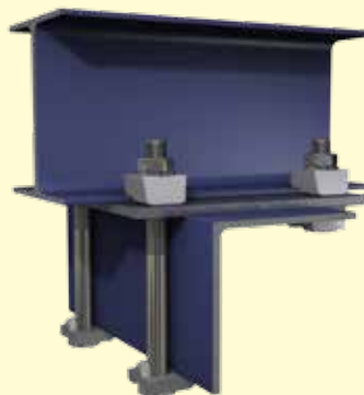
Angle section below an I-Section at 90 degrees
