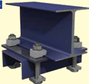
Channel section at 90 degrees below an I-Section
